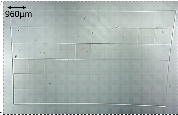
Figure 1: (a) arrays of 960x960 \mu\text{m}^2 developed in the photoresist using grayscale lithography; (b) one array after transfer into the Si substrate by plasma etching
